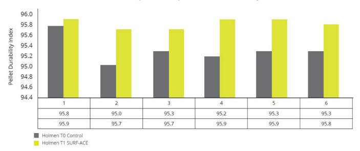
Pellets need to withstand significant pneumatic handling, for example, during bagging and transport, and in the feed lines. The Holmen durability tester simulates this handling, and calculates the percentage of fine generated, expressed as a pellet durability index (PDI). Across six different poultry compound feed types, SURF•ACE improves pellet quality and thus the PDI. Fewer fines equate to less reprocessing for feed manufacturers and higher palatability for animals.
