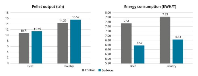
■ In Poland, another trial conducted at a commercial feed mill found that when SURF•ACE was added to 1% mixer-moisture, this lead to a 28.6 % higher feed throughput in the pellet press, 23 % lower energy consumption per unit produced during the pelleting process, and a nearly 1 %-point higher moisture content in finished feed. This resulted in higher profitability: based on the costs in Poland at the time of the trial, an ROI of 2.4:1 was achieved.
