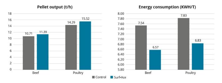
■ In Poland, another trial conducted at a commercial feed mill found that when SURF•ACE was added to 1% mixer-moisture, this lead to a 28.6 % higher feed throughput in the pellet press, 23 % lower energy consumption per unit produced during the pelleting process, and a nearly 1 %-point higher moisture content in finished feed. This resulted in higher profitability: based on the costs in Poland at the time of the trial, an ROI of 2.4:1 was achieved.
